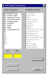
Fill in the **MIN** and **MAX** boxes to define the display scaling for that graph line. **Check** the **Auto Re-Scale** box for the y-axis to re-scale if the MIN or MAX value is exceeded. The MIN and MAX values will be used as the starting scales for that line on the graph.
