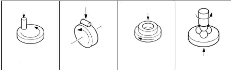
These are machines in which the point of contact is stationary with respect to one of the specimens and subject to constant speed uni-directional sliding. It is important to recognize that there are virtually no real life applications other than perhaps braking systems in which this occurs, thus introducing a degree of unreality to the test.
