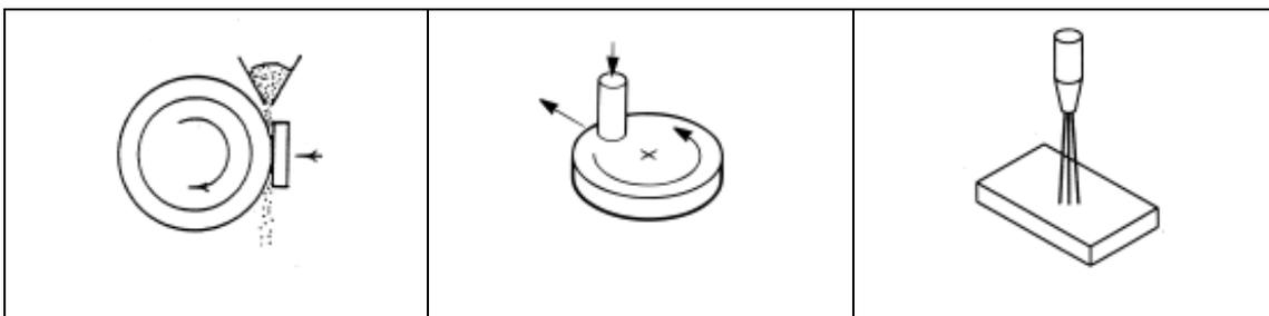
Abrasive and erosive testing of materials requires different types of machine from the primarily adhesive wear test machines discussed above, as a free body is usually involved. Although the size of test samples may be small compared with real life applications, satisfactory data can only be generated by matching conditions within the real life process, hence these are effectively “real life” and not scale model test devices.
