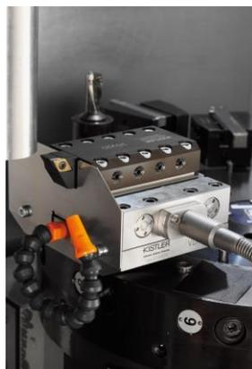
Kistler 3-axis Machine Tool Dynamometer
