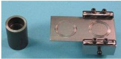
The tests demonstrate comparative performance between different lubricants and material combinations and the ability of these to prevent pick-up and galling under boundary lubrication conditions. Test duration can be used as a measure of lubricant squeeze film effects. Unlike the ring compression test, the twist compression test does not involve plastic deformation of the work-piece.
