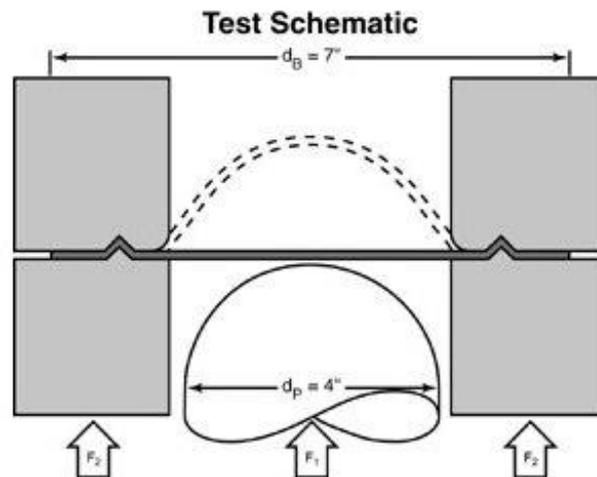
Schematic showing Tool and Specimen Dimensions for the Limiting Dome Height Test. Specimen after an increment of deformation is shown as dotted lines.
