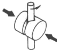
In the pin on vee block test, a load is applied to a pair of vee-notched jaws loaded on either side of a rotating pin, immersed in a test fluid sample. The test may either be run with progressively increasing load, in order to generate a scuffing failure, or under steady state load in order to measure wear. The machine is used extensively on neat oils (not emulsions), to evaluate extreme pressure additives.
