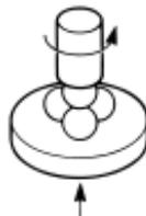
Both four ball wear and four ball extreme pressure tests have been used for evaluating metal working fluid performance.
