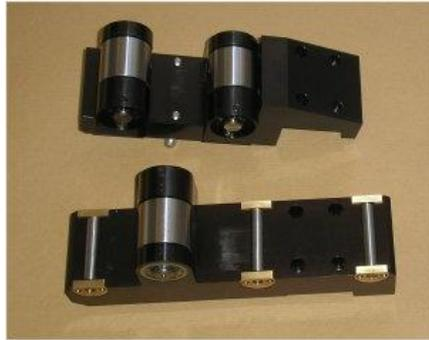
Fixed and rolling bead tests are performed with the same tooling and rollers. To convert from fixed roller bead to rolling roller bead, anti-rotation pins on the rollers are removed.
