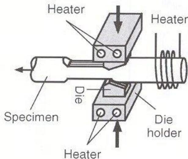
A range of heated Up-setting Tests have been used to model hot forging processes. This tests typically involve drawing a pre-heated rod sample through a die tool in much the same way as with a standard strip draw test. It is not clear whether anyone has thought of adapting the test to provide a similar method to the roller bead test.
