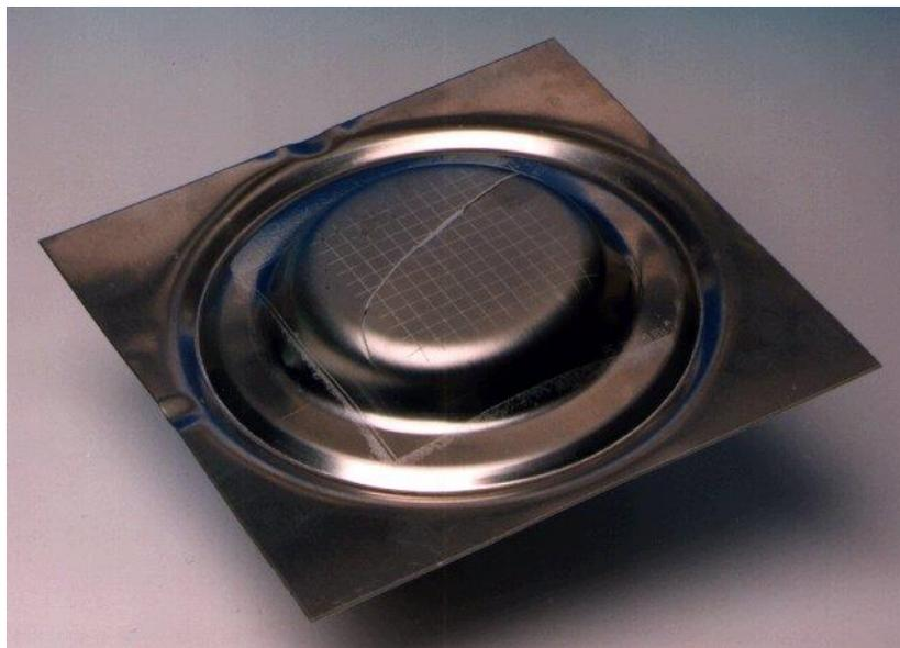
The tests can however be used to investigate a range of tribological properties including coating adhesion to the substrate in pre-coated sheet material, influence of lubricant pre-treatment on drawing force and the influence of tool design, surface finish and clamping force on "draw-in".
