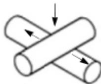
Finally, it would possible to devise tooling to allow one of the rollers to rotate, thus imposing combined sliding and rolling on the contact.
