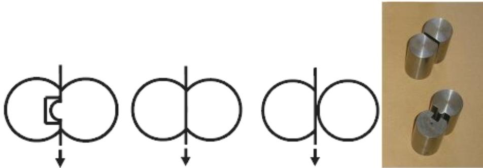
Strip draw tests using a range of flat face and bead die sets are used for evaluating the influence on frictional behaviour of lubricants, work piece materials and tooling coatings and surface roughness and to investigate the resulting surface finish on the work-piece. Such semi-industrial type tests produce generally good correlation with full scale applications.
