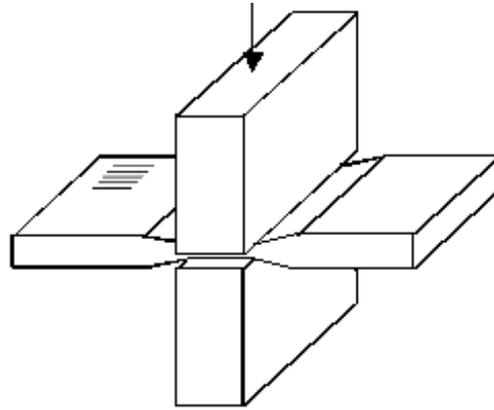
The plane strain compression test is used to estimate values of friction coefficient under boundary lubrication in rolling processes and to investigate the generation of fresh material and deformation and cracking of oxide films. Measurements of friction correlate with build up of transfer layers.
