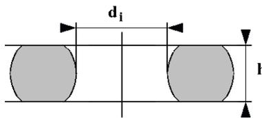
The ring compression test (Male and Cockroft – 1965) was developed to investigate the friction at the interface between a work-piece and a pair of platens. A flat ring shaped specimen is loaded between platens in a servo hydraulic test machine and subjected to axial compression. If there were no friction, the ring would increase in diameter radially with both the inner and outer diameters increasing.
