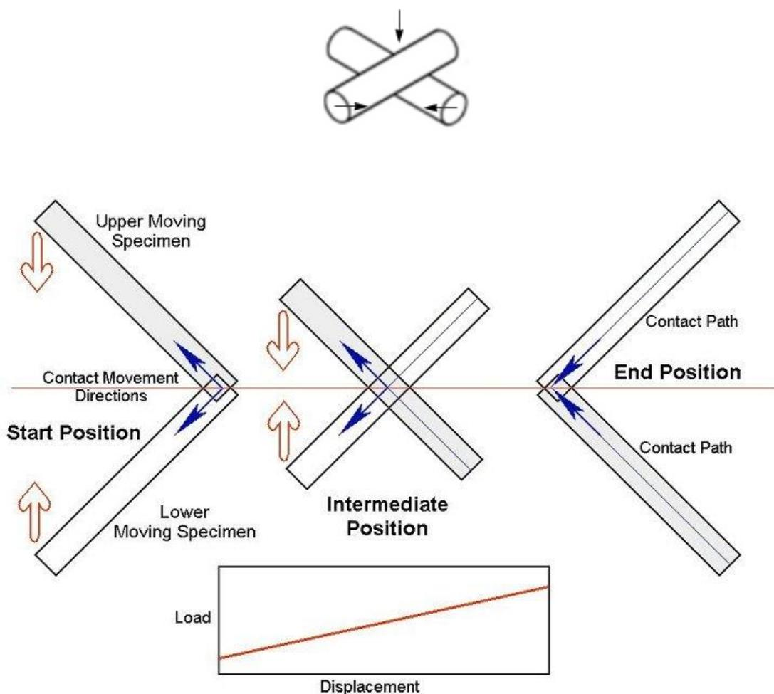
The load scanner is a concept developed by Professors Sture Hogmark and Staffan Jacobson at Uppsala University. The device offers a new test configuration for assessing the friction and wear properties of materials and lubricants. Two elongated test specimens, preferably bars or rods, are used. The orientation of the test specimens and their relative sliding motion during
