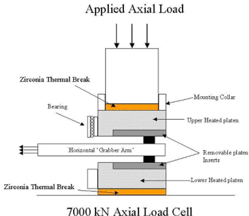
Friction coefficients are obtained from the rig by measuring the ratio of the horizontal load exerted by a hydraulic ram dragging a cylindrical billet across the face of two platens, compressed in a large 700 tonne press. Either 30 mm
