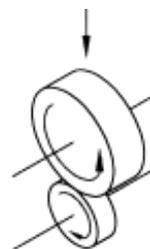
Two roller machines have been used for the investigation of the performance of lubricants in hydrodynamic, boundary and mixed lubrication regimes.
