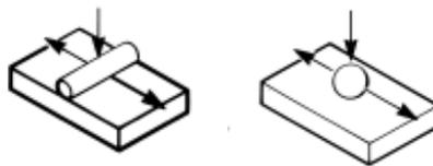
A number of users have attempted to model rolling processes using a long stroke reciprocating rig and claim to have generated some useful data. They found that because of the low frictional energy input to the contact, tests could be run under almost isothermal conditions.
