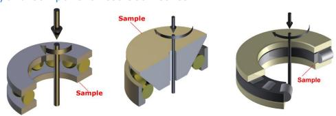
Hybrid Component Test Geometries
