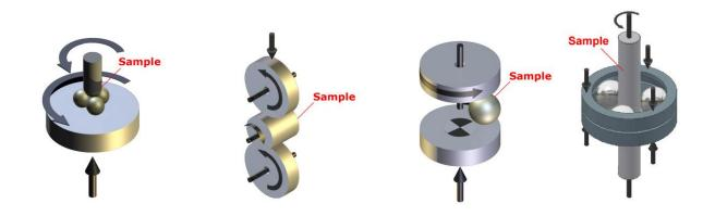
These tests are aimed at stressing a single rolling element component, either a ball or a rod. These tests are used for both material and lubricant tests.
