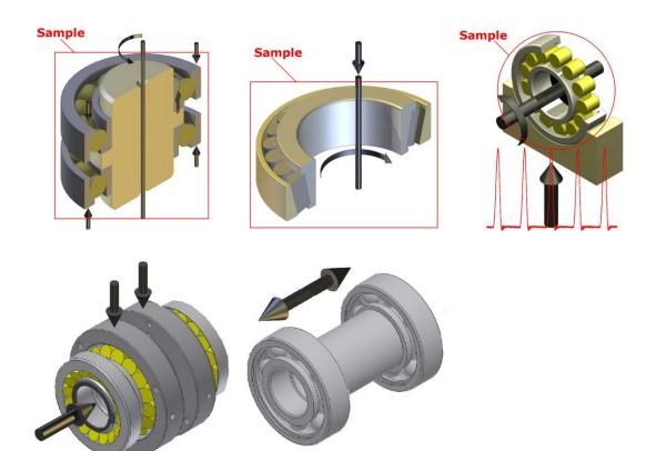
These tests use standard rolling element bearings as the test component. Tests may form the basis either for life testing the bearing itself or for evaluating the performance of a lubricant or grease.
