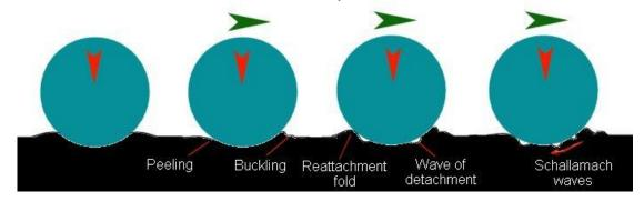
Under relative motion, "waves of detachment" form at the leading edge of the contact and flow across the contact area away from the leading edge. Rather than gross sliding over the complete contact area, the surface displacements move in folds or buckles. Before the rubber can buckle, it must first be peeled from the rigid counter-face and the energy required to do this generates significant frictional resistance.
