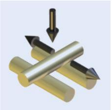
For practical purposes, it is easier to use a "pin on twin" geometry, with the "pin" the elastomer. This works if the pin is a thin sheet of rubber glued to a metal cylinder sample.
