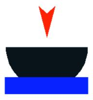
A thin disc of the same rubber material is made with exactly the same diameter as the contact area of the hemisphere under load. This is then subjected to the same applied load as the hemisphere. Care has been taken to support the disc in a holder to minimize the cantilever effect.
