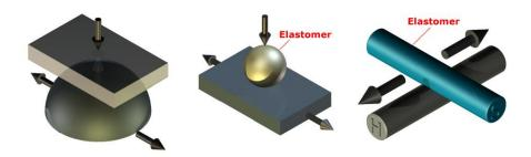
In addition to the more conventional test parameters: load, temperature, sliding speed etc, we found that a key variable for our tests was dwell time, both following the initial application of load and at the end of each stroke. Controlling the dwell time precisely had a significant impact on improving test repeatability and the instrument we developed included the means for controlling the application and removal of load.
