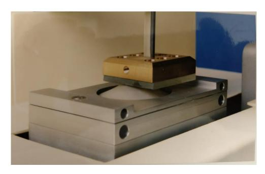
With this geometry, a flat counter-face surface is loaded against an elastomer sphere or hemisphere. This ensures a flat friction contact. In the example shown above, a thin sheet of elastomer (from a surgical gloves) has been stretched and clamped over a hemispherical elastomer hemisphere. In addition to modelling contacts between an elastomer and a hard surface, this geometry has also been used in skin friction simulations.
