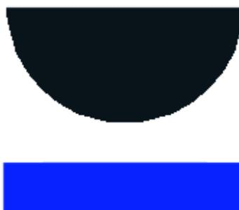
The rubber hemisphere is loaded into contact with the hard surface elastically, producing a given contact area.
