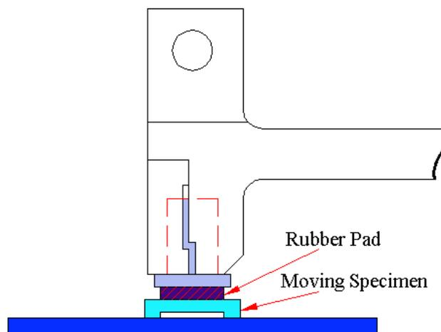
The stepped moving specimen allows the rubber layer to shear as opposed to acting as a cantilever, thus producing better defined contact conditions.
