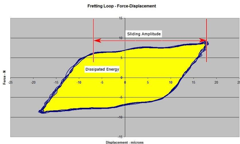
As the contact progresses from fretting (combined regimes of slip and non-slip) to bulk sliding, the shape of the loop changes.
