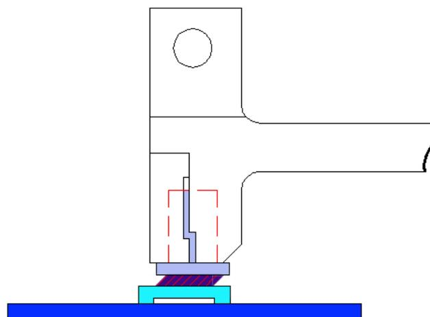
The stick-slip arrangement is ideally run at low sliding speeds and is thus run using the TE 77/GB20 or TE 77/GB100.
