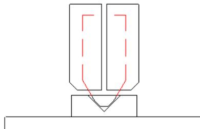
Another form of self-aligning arrangement is to use a hemisphere for the pin:
