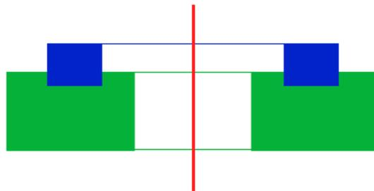
If the smaller upper specimen is softer than the larger diameter lower specimen, the edge effect is removed, but elastic deformation of the softer material may result in a change in apparent area of contact.
