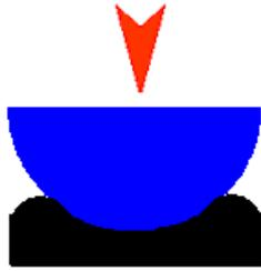
There are considerable problems with the hard ball on soft rubber flat test configuration, in both dry and lubricated sliding. The hard ball deforms the softer surface elastically and material relaxation occurs with time.
