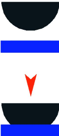
In this configuration the rubber sample is self-locating and issues of specimen alignment, fluid entrainment (in lubricated tests) and material hysteresis effects are minimized. The resisting force vector is fully deterministic and is generated by friction.
