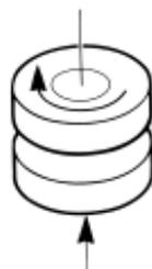
However, even with a continuous contact, edge effects must be considered, especially if one specimen has a smaller outer diameter and larger inner diameter than the other.
