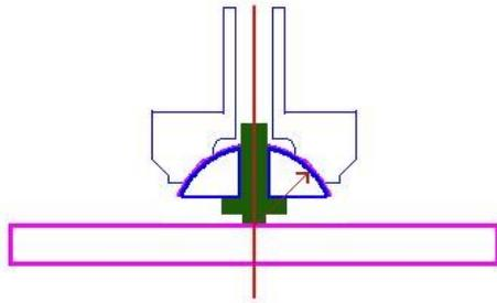
In both cases, the centre of the contact should be the centre for the spherical seat.
