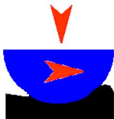
With relative sliding, a bow wave of material forms in the direction of sliding with a wake of recovering material left behind in the opposite direction. The vector of the resisting force is indeterminate and it is not exclusively generated by friction.
