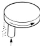
In this case, the debris may fall off the disc surface giving a different friction and wear performance compared with the previous case.
