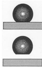
Measurement of material lost from the softer pin or ball is relatively easy. It should however be remembered that if material has been transferred to the disc or plate, its mass may increase.
