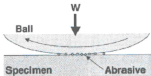
The contact in this case is now quite definitely operating in what is classically referred to as "three body abrasion", with the wear debris acting as the third body. However, the term "three body abrasion" is perhaps somewhat confusing and it should perhaps be referred to as "third body abrasion" for clarity.
