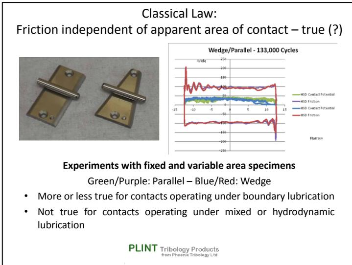
The law that states that friction is independent of apparent area of contact is more or less true for contacts operating under boundary lubrication.
