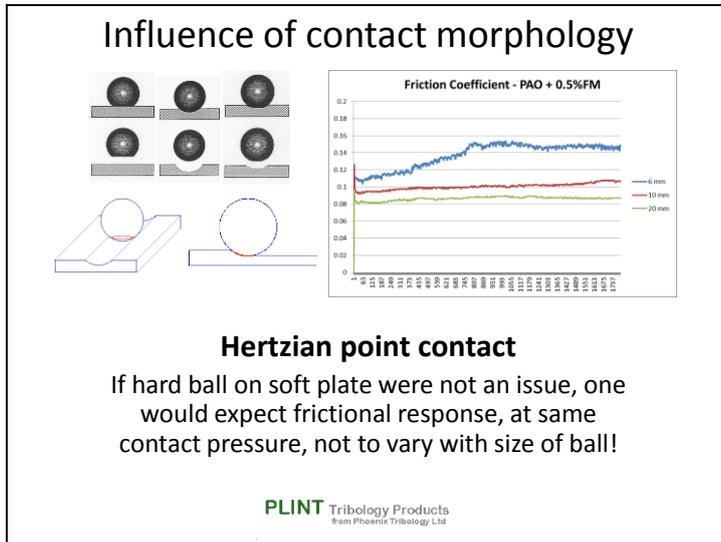
With a soft ball running on a hard surface, the contact patch remains flat and round; this is readily amenable to analysis of the forces acting on the contact. This is not the case with a hard ball sliding in a conforming wear groove on a softer surface.
