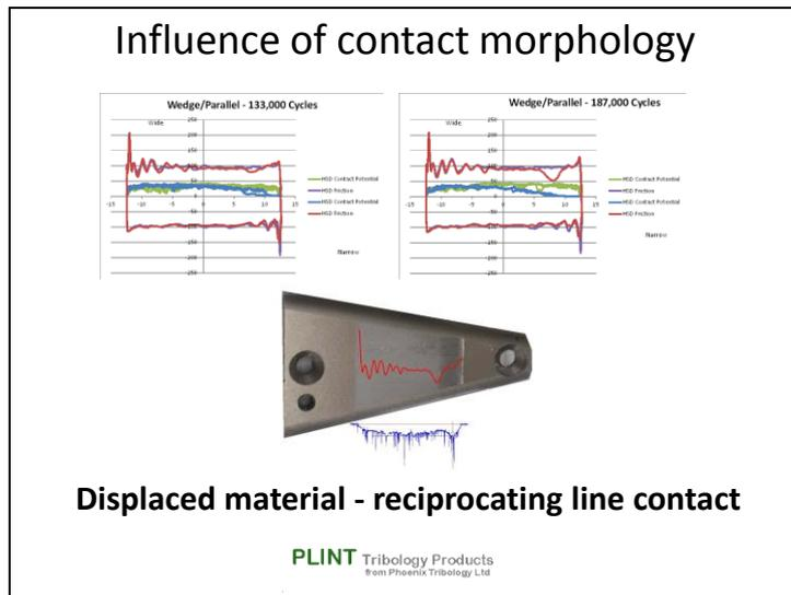
The dip in friction trace towards the stroke end, with the wedge specimen, is associated with a change in surface topography.
