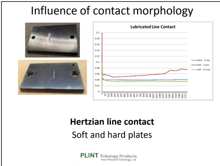
Similar effects can be seen with a cylinder on flat line contact. At short strokes the hard cylinder on soft plate can result in much higher friction than the same cylinder on a hard plate. In this example, with the former, a hole has been dug in the surface; with the latter, the contact patch remains essentially flat.
