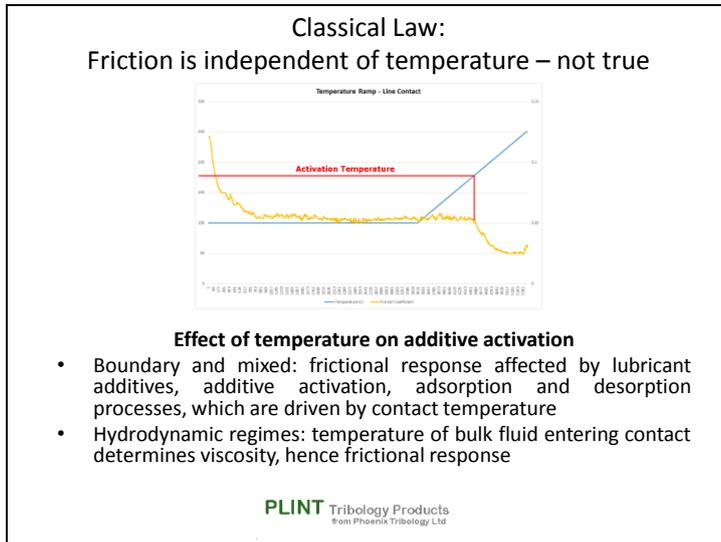
In a lubricated contact, friction is not independent of contact temperature.
