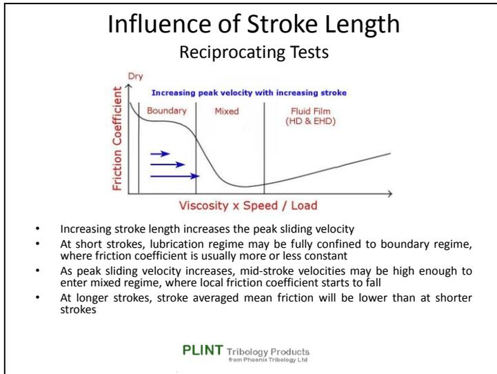
In exactly the same way that real contacts (gears, ring-liner etc) operate across lubrication regimes, the same happens with reciprocating tribometers.
