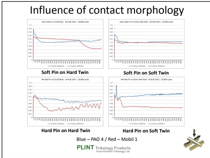
The pin on twin geometry provides very clear examples of the effect of wear track shape, resulting from a combination of contact geometry and relative specimen hardness, on frictional response.
