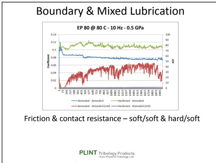
With a harden roller running on a soft plate, the hard roller abrades the softer surface producing a significant amount of oxide debris in the oil. The hard ground surface remains rough throughout, with friction levels typically associated with boundary lubrication. The ploughing (or two body abrasive) component of friction is dominant.
