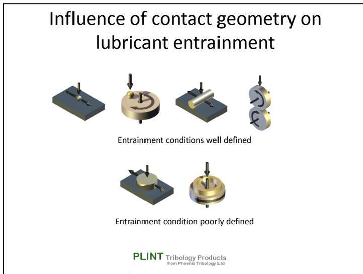
The different contact configurations for sliding or sliding/rolling tests affect lubricant entrainment in different ways.
