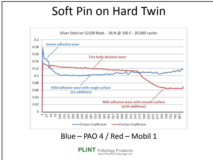
With the fully formulated oil, we observe mild abrasive wear transitioning to mild adhesive wear.
