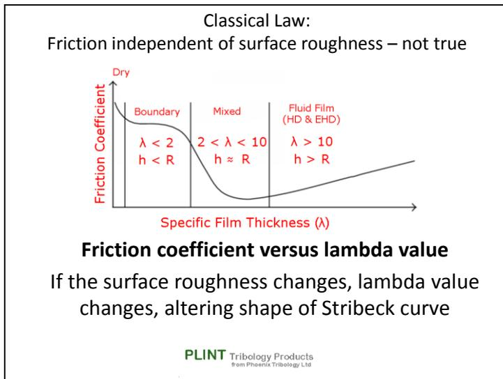
Friction is not independent of surface roughness.
