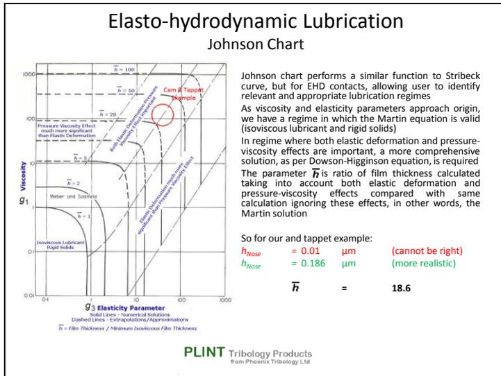
In 1970, Johnson introduced the concept of the “Johnson chart”, which performs a similar function to the Stribeck curve, but for EHD contacts. This allows the user to identify relevant and appropriate lubrication regimes.
