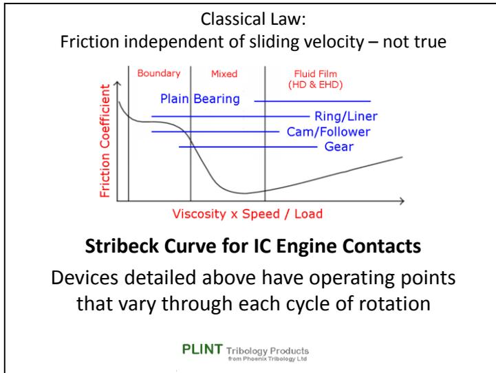
In a lubricated contact, friction is not independent of sliding velocity.
