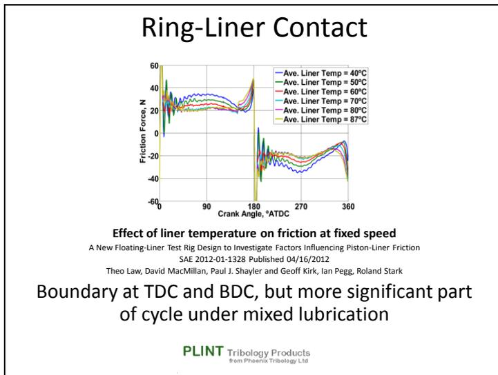
In the ring-liner contact, for example, although the contact may be running under boundary lubrication at top and bottom dead-centre, a more significant part of the cycle may be operating under mixed lubrication conditions.
