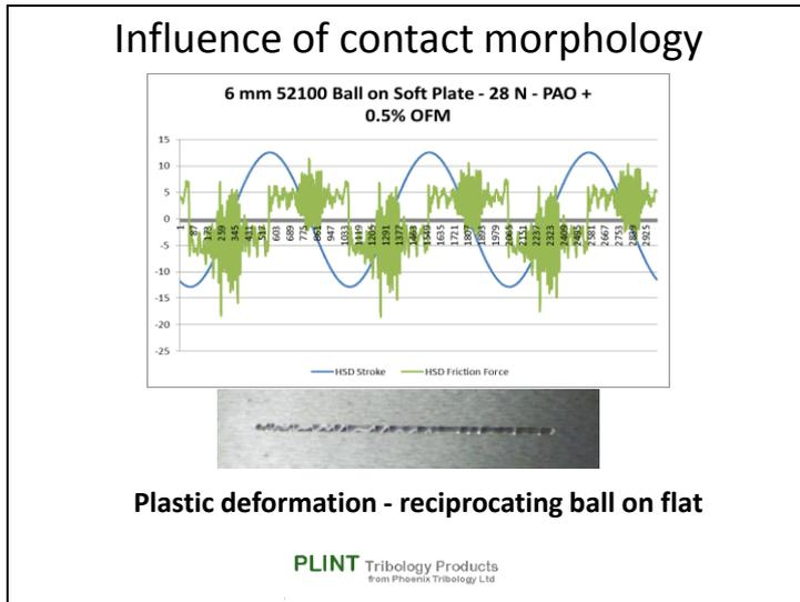
How a given contact wears or deforms depends on the relative hardness of the specimens. The shape of the resulting wear track affects the frictional response.
