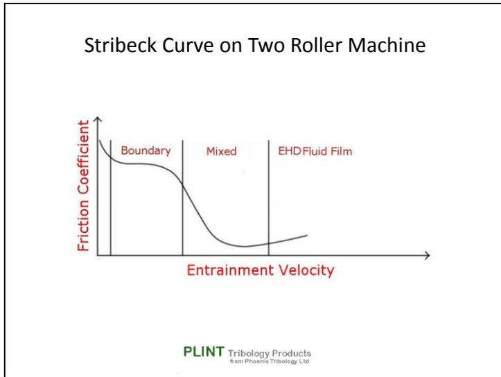
The friction or traction coefficient plotted against entrainment velocity.
