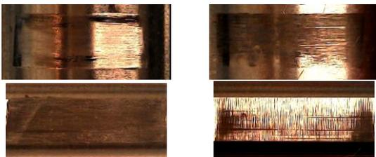
**Hard roller on soft flat**      **Soft roller on soft flat**
