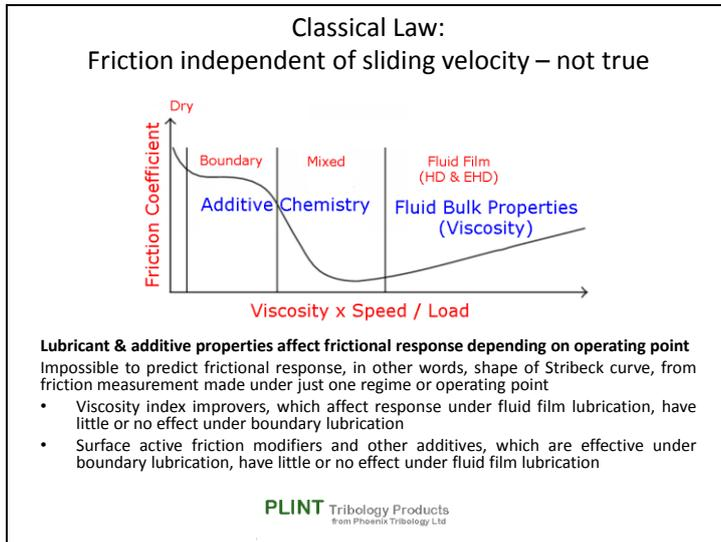
Lubricant and additive properties affect frictional response, depending where we are on the Stribeck curve.
