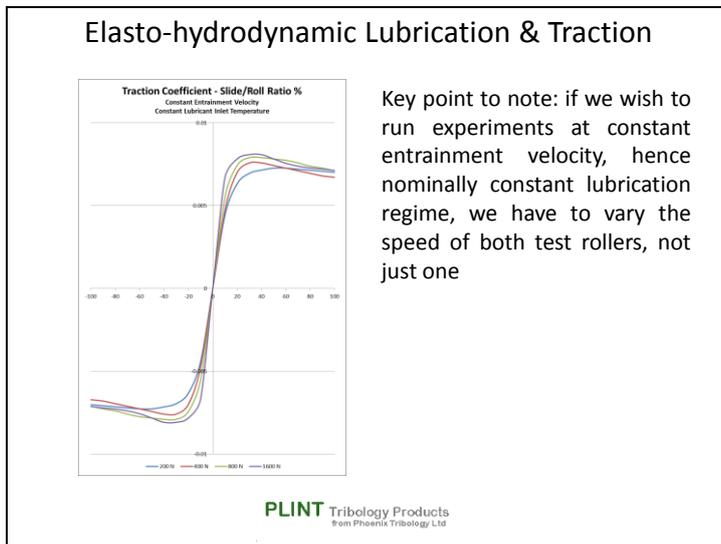
A key point to note is that if we wish to run experiments at constant entrainment velocity, hence nominally constant lubrication regime, we have to vary the speed of both test rollers, not just one.
