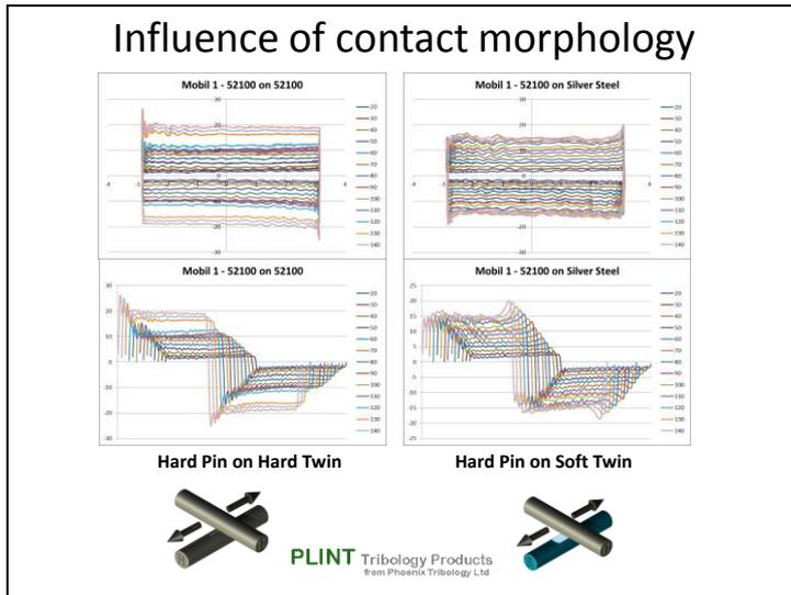
Differences in the shape of the friction loop/instantaneous friction signal for hard on hard and hard on soft illustrates the effects of contact morphology on frictional response.
