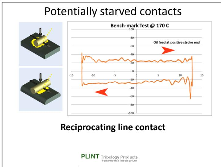
It is possible to produce an asymmetrical contact in a reciprocating test, by not allowing the lubricant to spread to both sides of a line contact. This produces starved lubrication in the sliding direction away from the lubricant feed and fully flooded lubrication in the opposite direction, hence different regimes, depending on the direction of sliding, hence a direction dependent frictional response.
