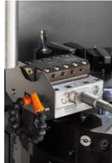
Kistler 3-axis Machine Tool Dynamometer
