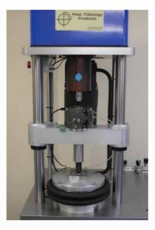
The high load actuator assembly is used in conjunction with the back-to-back bearing assembly and allows loads of up to 40 kN to be applied to the test bearings and a maximum rotational speed of 10,000 rpm to be achieved.
