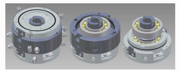
This adapter uses two size 7209 85 mm O/D 45 mm I/D angular contact bearings, loaded back to back, as the test samples. Separate oil ways are provided to ensure that oil and wear debris from the upper test bearing does not pass through the lower bearing.
