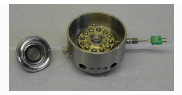
This adapter uses one half of a standard size 51208 68 mm O/D 40 mm I/D thrust bearing, with the balls running between the normal bearing race and a flat disc. A cage is provided to retain the balls.
