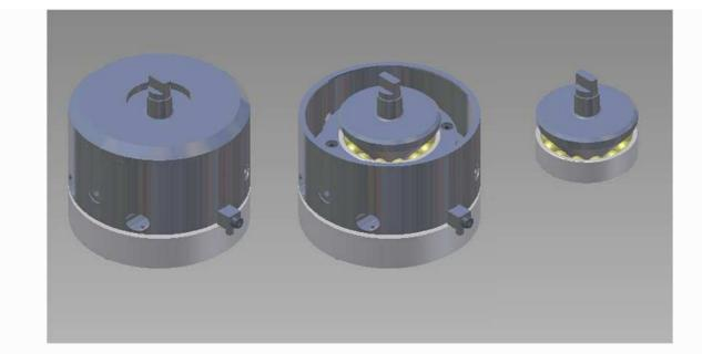
This adapter uses a conical test sample loaded against the lower half of a size 7206 62 mm O/D 30 mm I/D angular contact bearing. The cone angle is designed to give a pure rolling contact. Contact stress can be increased further by removing balls from the bearing cage.
