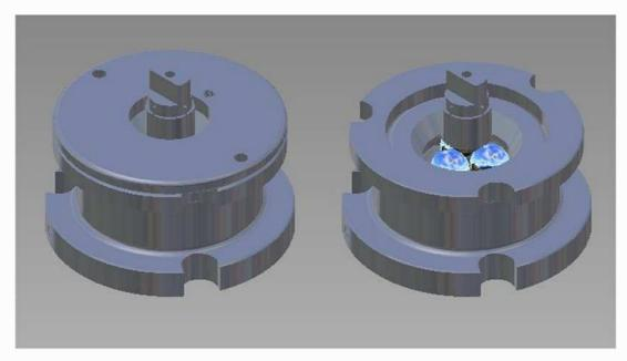
This comprises a test reservoir and precision polished test race. The race is designed to permit the test balls to rotate freely maintaining a defined contact angle with the upper ball fixed in the spindle.
