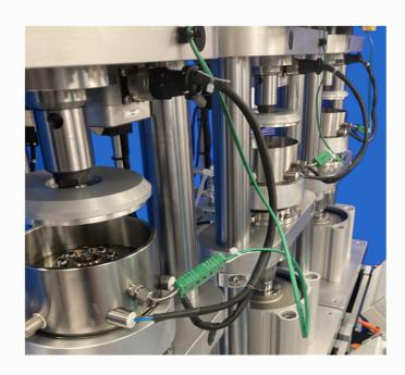
The machine is floor standing and designed to be installed either as a single unit or, more cost effectively, as a multi-unit installation, using a common lubricant service module and with the same pneumatic load applied to each test station.
