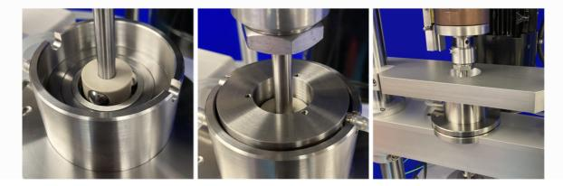
The machine is floor standing and designed to be installed either as a single unit or, more cost effectively, as a multi-unit installation, using a common lubricant service module and with the same pneumatic load applied to each test station.
