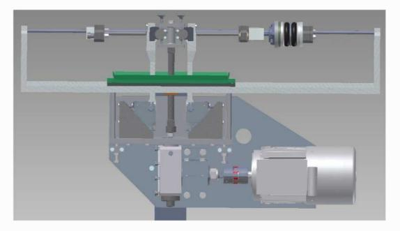
Load is applied to either side of the moving specimens by squeezing the two fixed specimen arms together by means of a servo controlled pneumatic bellows assembly, with force transducer feedback. This arrangement ensures that there is no bending moment acting on the moving specimen carrier.
