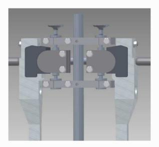
Various tooling options are available in addition to conventional point, line and area contact configurations. Current options include valve stem and valve guide fixtures, and piston ring against cylinder liner. In this latter configuration, a complete piston ring is loaded against a segment of cylinder liner and means are provided for closing the ring gap and for tilting the ring relative to the liner, thus facilitating conformity and alignment.
