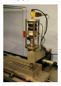
A strain gauge load cell is mounted at the rear of the pin carrier block, preventing the block pivoting about its central axis. This transducer therefore measures the force exerted on the pin during sliding. A retaining clamp maintains the pin carrier in contact with the transducer at all times, ensuring that bi-directional forces generated in pin on disc and reciprocating contacts are measured.
