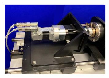
For oscillating motion of  $+/-20^{\circ}$  at 1 Hz, the direct drive motor is replaced with a smaller servo motor driving through a 100:1 reduction gear-box.
