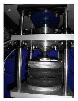
A force transducer is included for measurement and feedback of load, for servo pneumatic control.
