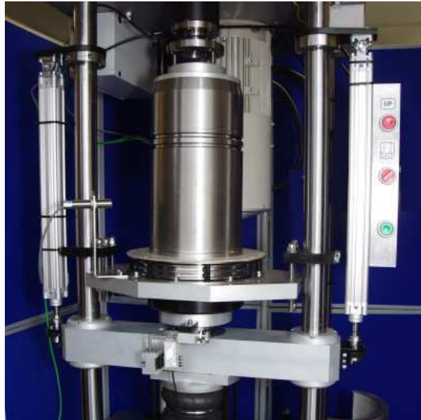
Large diameter liner in place
