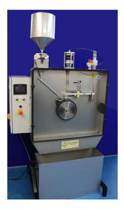
For wet tests, water is introduced on to the wheel surface, just behind the chute. This means that fully wet tests can be carried out, with the mass flow of abradant still controlled. This is not possible in the ASTM configuration.
