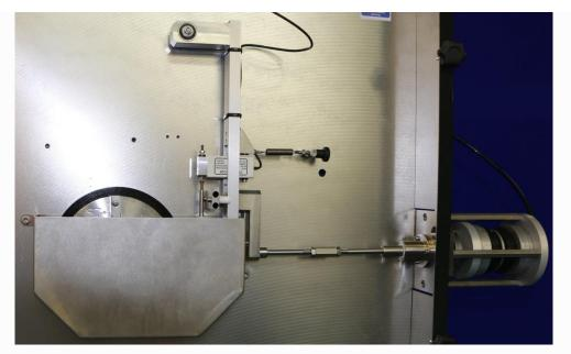
The TE 65 includes the option of a second loading system that presses the specimen on to the top of the wheel, with the specimen horizontal.
