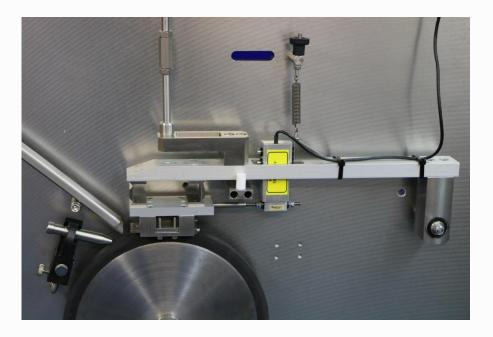
The alternative abradant feed system is designed to give a range of constant feed rates and produce an even monolayer of particles on the wheel in front of the contact. The abradant is fed from a hopper to a rotating drum with a shallow groove on its surface. The feed rate is varied by adjusting the speed of the slotted drum. The out-fall from the drum is then guided to the wheel surface down a simple chute and this produces the monolayer on the wheel surface.
