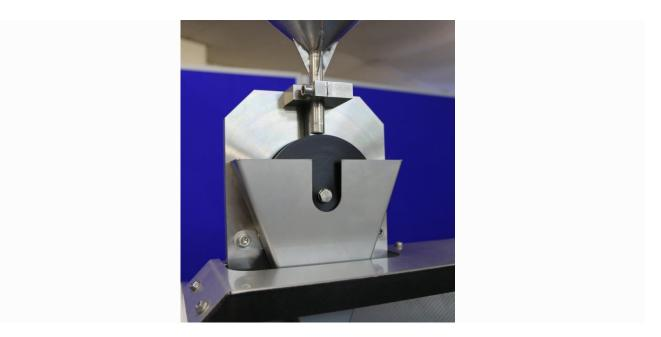
Any abradant that does not pass through the contact may be collected separately and therefore the quantity of abradant actually passing the test block may be determined. This is not possible in the ASTM configuration. By having control of the drum speed, much lower abradant mass flow rates can be achieved than in the ASTM G 65 method.
