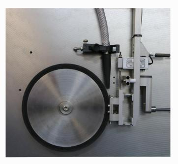
The other standards have a fluid trough and the slurry is agitated by the wheel rotation. ASTM B 611 uses a steel wheel, thus providing higher stress abrasion than the rubber wheel tests.
