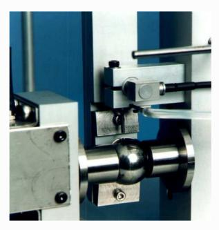
This non-contacting displacement transducer may be used to monitor the position of the beam relative the ball axis during a test. Wear depth and wear rates may be determined from this measurement. The use of the TE 66/W system is recommended only for tests where the coating or substrate will be wearing more than 10  $\mu$ m.
