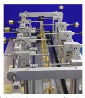
In addition to the standard single station tester, multi-station units can be assembled, incorporating a single drive motor and control system and multiple test assemblies. This is an economical way of increasing testing capacity without increasing the number of testers required.
