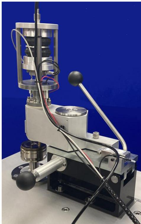
A strain gauge load cell is mounted at the rear of the pin carrier block, preventing the block pivoting about its axis, hence sensing the friction force exerted on the pin. The low rotational inertia of the carrier block about this axis ensures a good signal bandwidth for the friction measurement.
