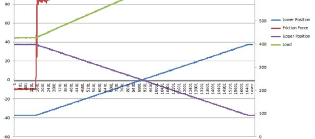
The relative motion is generated by two servo-controlled ball-screw actuators, with one connected to the lower specimen carriage and the other to the upper specimen carriage. The carriages are moved synchronously, in equal but opposite directions, so that the point of contact does not move relative to the machine.
