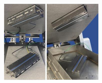
Tests may be run either dry, with the rod samples carried on individual heater blocks, or lubricated, with the lower rod sample carried in a heated lubricant bath.
