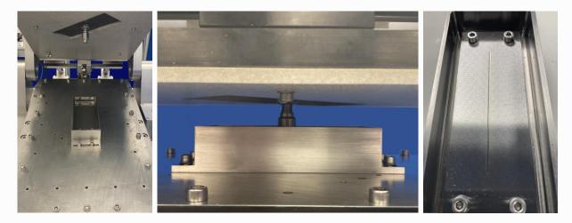
Independent control of the load allows tests to be run with a steady state load, or with a ramped load as in a conventional scratch test.
