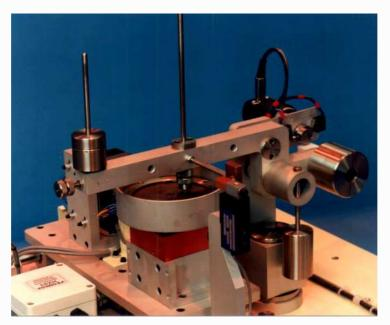
This Module comprises a rotating disc assembly mounted on a cross slide, thus allowing the pin sample to follow a spiral track on the disc, if required. Rotary and translatory motions are driven by stepper motors. The module locates on the base plate of the TE 79 Base Unit and is fixed in place with locating screws.
