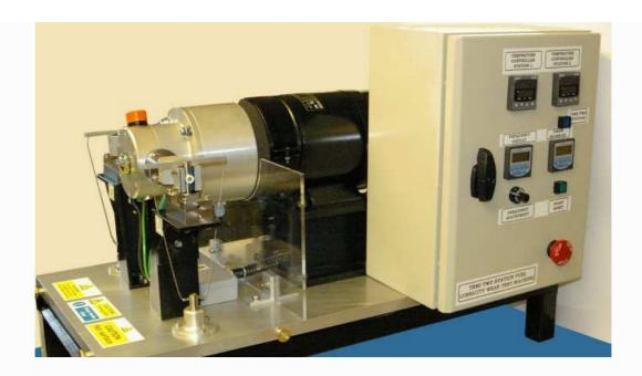
The TE 80 Fuel Lubricity Tester will run tests in accordance with the test parameters specified in ISO 12156-1 and ASTM D6079 fuel lubricity test standards and will rank fluids in the same order, but will consistently produce larger wear scars than the PCS HFRR instrument and a wider discrimination between low and high reference fuels.
