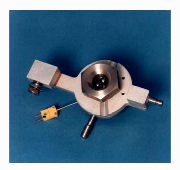
The TE 82 includes the test adapter for sliding four ball tests. This comprises a test reservoir, clamping nut, thrust face and clamping ring for the three test balls, integral torque arm and thermocouple sensor.
