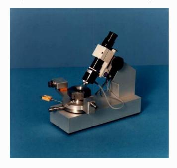
The TE 82/SCOPE High Resolution Microscope Assembly provides for rapid measurement of the wear scar on the test balls from a sliding four ball test (EP or Wear) without having to removing the balls from the sliding 4-ball test adapter.
