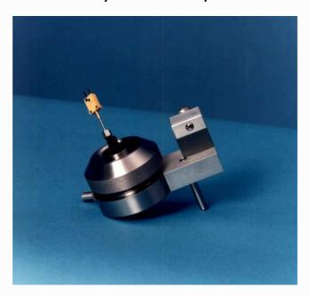
The DIN 51350-6 and CEC test methods are for the determination of the shear stability of lubricating oils with polymer additives. For this a taper roller bearing is used to shear the fluid. The purpose of the test is to determine the permanent drop in viscosity caused by mechanical stresses under practical conditions.
