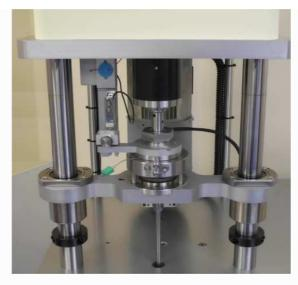
Vector control of the motor with encoder feedback provides a variable speed turn-down ratio of 100:1. The motor is four-pole providing a constant torque of 14 Nm up to 1,500 rpm and constant power of 2.2 kW from 1,500 to 2,000 rpm. The motor is capable of providing 50% overload for 30 seconds and therefore a maximum torque of 21 Nm is available for this time. The welding limit in 4-ball EP tests is typically 12 Nm.
