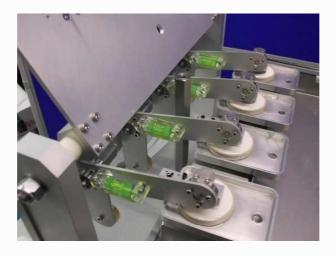
Teeth samples, which are normally set in epoxy discs, are held in radially sprung fixtures.
