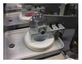
Load is applied directly to each toothbrush sample by dead-weights acting on linear bearing mounted load rods.
