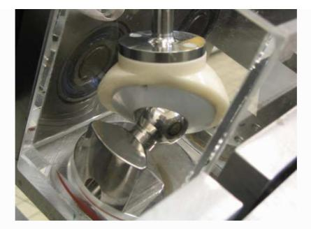
An acrylic lubricant chamber with a volume of 500 ml fits over the test components. The fluid volume is deliberately large in order to eliminate the possibility of overheating of serum-based lubricants.
