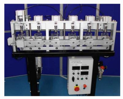
The two-axis motions, flexion-extension (FE) and abduction-adduction (AA), are nearly sinusoidal, and their phase difference is pi/2. As internal-external rotation has been shown to be unimportant in the simulation of clinical wear, this motion has been excluded.
