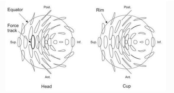
The force track on the femoral head is elliptical with an aspect ratio of 3.8, which has been shown to be a good representation of human gait. The length of the force track is 1.73r, where r is the head radius.
