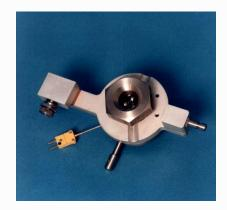
This comprises a test cup, clamping nut, thrust face, clamping ring, torque arm and thermocouple sensor. The upper ball is placed in a split taper collet, which is a push fit into the spindle taper.
