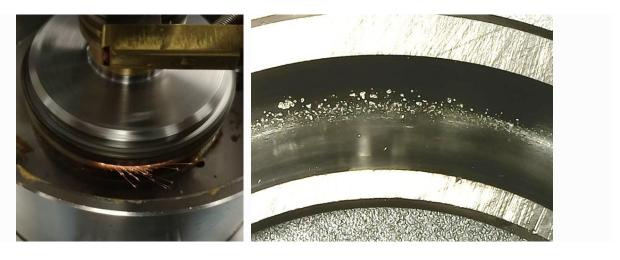
Non-electrically conducting bearing cages are used and other electrical isolation components are necessary and are incorporated in TE 92/RCF/2/E Ball Thrust Bearing Tooling for EDM Tests and TE 92/RCF/3/E Roller Thrust Bearing Tooling for EDM Tests.
