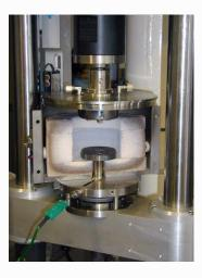
The TE 92/HT 600°C incorporates an electrically heated furnace. To ensure that heat conduction to the test spindle bearings is minimised, the machine is manufactured with a longer test spindle and therefore larger frame. This option is not available as a retrofit item and must be specified at the time of order. The adapter is suitable for dry tests in three rotating pin on non-rotating disc.
