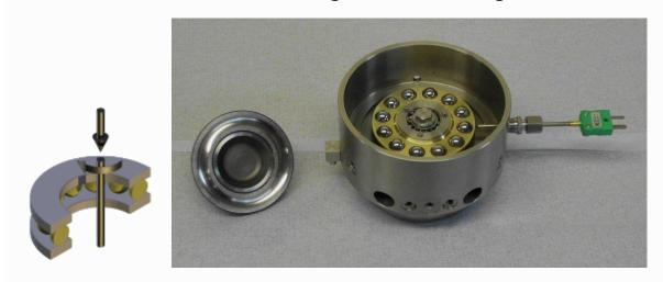
This adapter uses one half of a standard size  $51208\ 68\ mm\ O/D\ 40\ mm\ I/D$  thrust bearing, with the balls running between the normal bearing race and a flat disc. A cage is provided to retain the balls.
