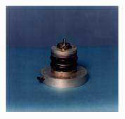
The TE 92/1 provides a loading range of 20 to 1,000 N and this is used for pin on disc, thrust washer and 4-ball wear tests.
