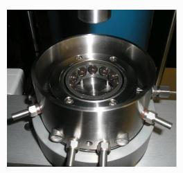
This adapter uses the lower race and cage of a standard angular contact bearing (SKF 7206), with the inner race replaced by a conical specimen. The cone angle is such that the rolling contact is pure rolling with no spin. With silicon nitride balls in the bearing race, contact pressures up to 5.5 GPa can be achieved. The cone is subjected to the highest number of contacts and thus it is the rolling fatigue performance of the cone material that is investigated in this test configuration.
