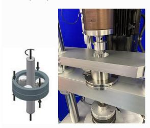
This adapter is designed to run the standard three ball on rod rolling contact fatigue test geometry, in which three balls, separated by a retainer, are loaded against a rotating rod specimen, by applying an axial force across two taper bearing cups, mounted above and below the three balls. The original design, dating from the 1970s, used pre-set compression springs to apply the axial load; in this application, the axial load is generated using the **TE 92/1 Low Load Actuator**.
