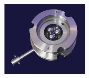
This comprises a test reservoir and precision polished test race. In this case there is no torque measurement. The adapter may be used in conjunction with **TE 92/2 High Load Actuator** to perform tests in accordance with:
