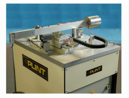
The fixed plate specimen is located on two screw fittings in a stainless steel reservoir. The reservoir is clamped to a block that is heated by electrical resistance elements and the temperature is monitored by a thermocouple pressed against the side of the specimen or holder. The reservoir can be moved sideways on the heater block so that multiple tests can be performed on one plate specimen.
