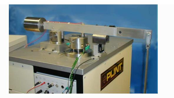
The test disc is mounted on the disc carrier spindle and secured by a central bolt. The spindle is driven through a pulley belt by the vector controlled a.c. motor mounted beneath the machine. The motor has encoder feedback to ensure stable running speeds.
