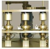
This machine is designed to run multiple tests in the thrust washer and three pin on disc test configurations, under identical test conditions. Sensors are provided for measurement of friction and sample temperature on each test station.
