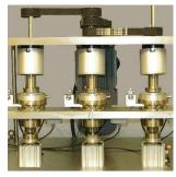
This machine is designed to run multiple sliding four ball friction and wear tests, under identical test conditions. Sensors are provided for measurement of friction and sample temperature on each test station.
