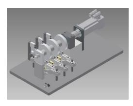
This wear and friction test machine uses simple test specimens offering conforming and non-conforming block-on-ring contact geometry. The machine meets and exceeds the requirements of ASTM G 137. Relocating block specimen holders provide for accurate re-positioning of the specimens after weighing: this enables wear to be measured during tests.
