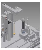
This is a three station version of the standard TE 66 Micro Scale Abraion Tester and is used to determine the wear coefficient of hard and soft coatings and monolithic materials by abrasive wear in a ball on plate contact configuration, in accordance with BS EN 1071-6. The instrument may also be used as a crater-generating tool on coated surfaces for coating thickness determination.
