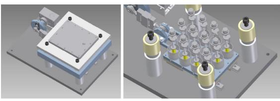
Load is applied to each test station by means of pneumatic cylinders, connected in parallel. Pressure to the cylinders is manually controlled by means of a precision pressure regulator.
