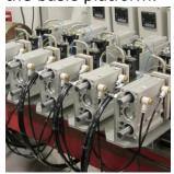
Load is applied to each test station by means of pneumatic cylinders, connected in parallel. Pressure to the cylinders is manually controlled by means of a precision pressure regulator.
