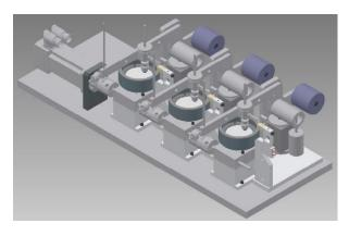
This unit incorporates three conventional pin on disc test assemblies, generally in comliance with ASTM G99.
