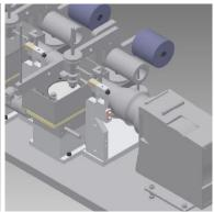
This unit incorporates three conventional pin on disc test assemblies, generally in comliance with ASTM G99. It is designed for running dry pin on disc tests at temeorature from ambient to  $500^{\circ}\text{C}$
