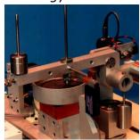
The unit incorporates three conventional pin on disc test assemblies, generally in comliance with ASTM G99.
