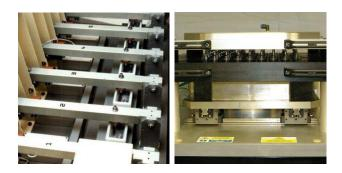
Load is applied to each test station by means of pneumatic cylinders, connected in parallel. Pressure to the cylinders is manually controlled by means of a precision pressure regulator.
