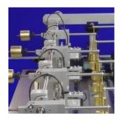
The unit is used to determine the wear coefficient of hard and soft coatings and monolithic materials, by abrasive wear, in a ball on plate contact configuration, in accordance with BS EN 1071-6. The instrument may also be used as a cratergenerating tool on coated surfaces for coating thickness determination.
