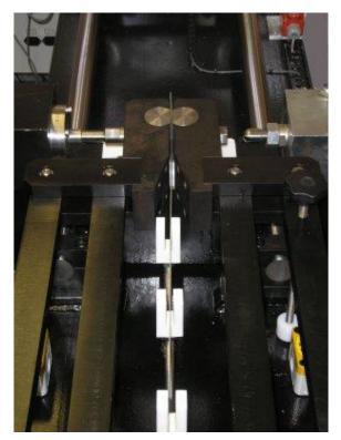
A variety of different tools may be used, providing a range of different sliding contacts including flat on flat area contact, cylinder on flat line contact and draw bead contact. In all these configurations, the friction force measured is the combined force on both surfaces. An alternative cylinder on flat line contact configuration is available in which the cylindrical tool is replaced by a roller, allowing sliding on one surface and rolling on the other.
