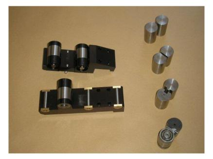
A roller bead test assembly is also available in which the rollers may either be unclamped and allowed to roll freely, thus generating only the deformation force, or clamped, thus generating combined deformation and sliding friction force.
