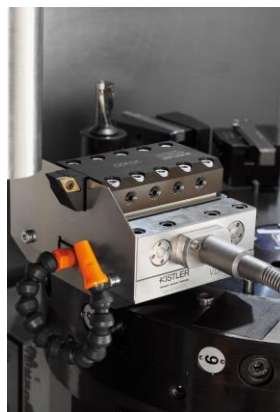
Kistler 3-axis Machine Tool Dynamometer
