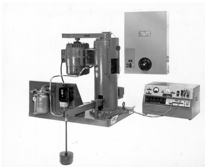
Original 30,000 rpm high speed rolling four ball machine
