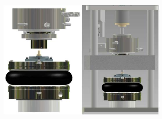
Load on the test bearing is reacted by a ball thrust bearing mounted on the underside of the machine spindle housing, thus ensuring loads are not reacted by the machine spindle bearings.
