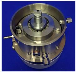
Custom bearing tooling is not included and must be ordered separately, to meet the user's specific requirements. The maximum bearing O/D that can be accommodated is 60 mm.
