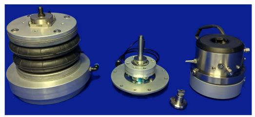
Load on the test bearing is reacted directly by the machine spindle bearings.
