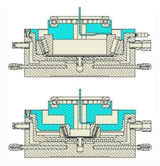
Custom bearing tooling is not included and must be ordered separately, to meet the user's specific requirements. The maximum bearing O/D that can be accommodated is 180 mm.
