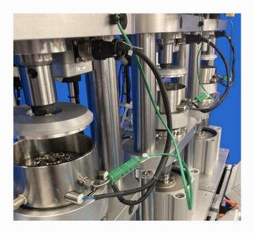
The machine is floor standing and designed to be installed either as a single unit or, more cost effectively, as a multi-unit installation, using a common pneumatic loading system, so that the same load is applied to each test station.
