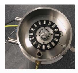
This adapter is essentially similar to RCF 5/1, but uses one half of a standard size 81208 TN roller thrust bearing, loaded against a flat lower disc sample, of chosen material. The standard bearing cage is used to locate the rollers, with the cage centred by a spindle mounted deep groove ball bearing.
