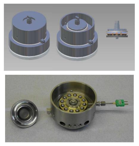
This adapter uses one half of a standard size 51208 68 mm O/D 40 mm I/D thrust bearing, with the balls running between the normal bearing race and a flat disc. A cage is provided to retain the balls.
