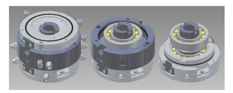
This adapter uses two size 7209 85 mm O/D 45 mm I/D angular contact bearings, loaded back-to-back, as the test samples. Separate oil ways are provided to ensure that oil and wear debris from the upper test bearing does not pass through the lower bearing.
