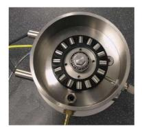
This adapter is essentially similar to RCF 7/1, but uses one half of a standard size 81208 TN roller thrust bearing, loaded against a flat lower disc sample, of chosen material. The standard bearing cage is used to locate the rollers, with the cage centred by a spindle mounted deep groove ball bearing.
