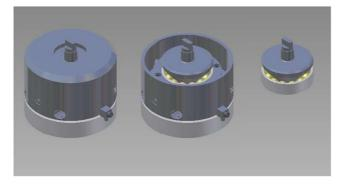
This adapter uses a conical test sample loaded against the lower half of a size 7206 62 mm O/D 30 mm I/D angular contact bearing. The cone angle is designed to give a pure rolling contact. Contact stress can be increased further by removing balls from the bearing cage.
