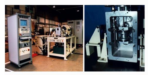
High Power (150 kW) Hydraulic Pump Test Rigs
