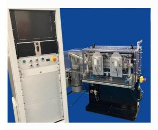
High Power (2 x 75 kW) High Speed (6,000 rpm) Two Roller Machines
