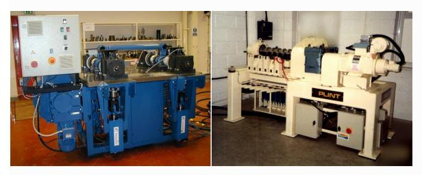
Full-scale, Back-to-Back, Gear-box Test Rigs
