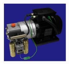
This unit, designed for SwRI, clearly demonstrated the superiority of a line contact fuel lubricity test over a point contact test, but who cares, if the ASTM standard specified a point contact?
