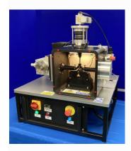
This was essentially designed to demonstrate that you do not need to use an expensive electromagnetic oscillator to run numerous ASTM standard ball on flat tests; you can get comparable results with a simple mechanically driven machine.
