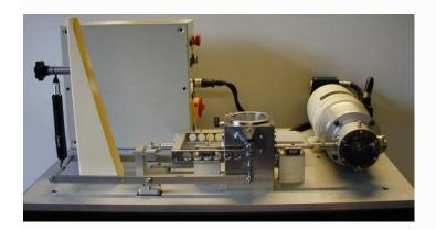
This unit has resulted in the generation of numerous well-received papers on refrigerant lubricants. The spring loading is antiquated and the specimen mounting is clumsy, however, the basic concept of applying load and measuring friction through bellows in shear is sound. The concept has been re-cycled into the recently designed adapter for TE 77.
