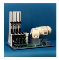
Designed exactly to meet the requirements of ASTM G137 Standard Test Method for Ranking Resistance of Plastic Materials to Sliding Wear Using a Block-On-Ring Configuration, the unit worked as required.
