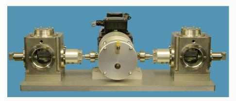
This was a spin-off from the TE 57 design and was used for testing the lubricity of volatile fuels such as DME, which requires a pressurised test chamber. It may be that with DME likely to be part of any future green fuel mix, pressurised testing may become of interest again.
