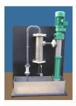
The particle amplifier design worked well, but it is difficult to make something like this look anything more than a piece of plumbing. Sure, the design can be improved, but it is still going to be large, cumbersome and dirty to operate. Perhaps there are no neat solutions to free-jet slurry erosion testing.
