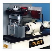
This was our version of a Japanese standard test for investigating frictional welding between piston ring and cylinder groove.
