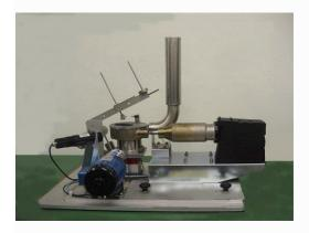
Designed to provide a simple 500°C pin on disc machine and based on TE 79, this is now an option on TE 79, as opposed to a free-standing instrument.
