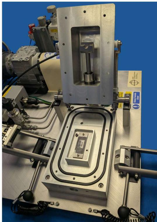
For access to the specimens, the pneumatic cylinders are folded to the side and the chamber fixing screws removed. The moving specimen arm and the chamber lid are then rotated together, out of contact with the chamber base.
