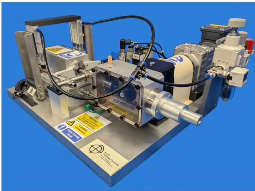
Reciprocating motion is generated using a scotch yoke drive from a standard TE 77 machine, driven by a gear-motor.
