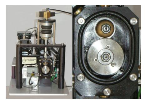
The ball-on-roller arrangement eliminates any possibility of spin or skew in the rolling contact and eliminates any uncertainty with regard ball or track diameter. With circumferential grinding of the roller, it eliminates all the an-isotropic materials properties associated with preparing the specimens.
