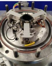
The test assembly, comprises three ball or line contact fixed specimen carrier assemblies, mounted on the top of the pressure vessel. A reciprocating drive projects upwards between the fixed specimen carriers and has locations for three plate specimens.
