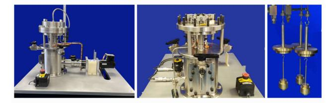
Reciprocating motion is generated by a manually adjusted, variable stroke, crank mechanism, a lower chamber. This is driven by an externally mounted, ATex rated, geared servo motor, via a magnetic coupling.
