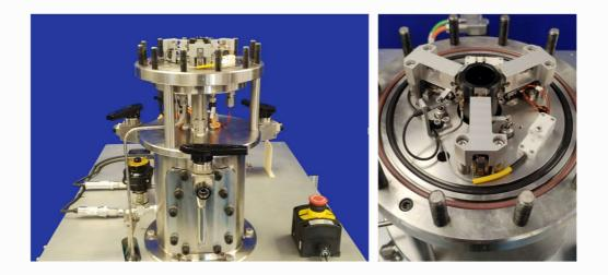
The test assembly, comprises three ball or line contact fixed specimen carrier assemblies, mounted on the top of the pressure vessel. A reciprocating drive projects upwards between the fixed specimen carriers and has locations for three plate specimens.
