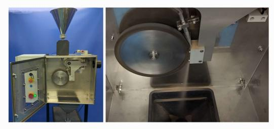
Enhanced control of the particle flow rate is achieved by the addition of a precision feed system.
