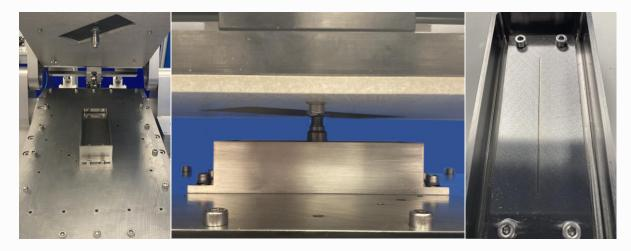
Independent control of the load allows tests to be run with a steady state load, or with a ramped load as in a conventional scratch test.
