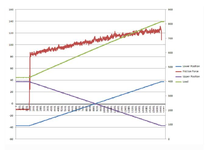
The relative motion is generated by two servo-controlled ball-screw actuators, with one connected to the lower specimen carriage and the other to the upper specimen carriage. The carriages are moved synchronously, in equal but opposite directions, so that the point of contact does not move relative to the machine.
