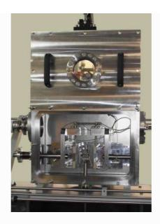
The test assembly is located vertically above the reciprocating drive assembly and comprises two fixed specimen pads, each mounted on flexures, with movement in the friction direction resisted by piezo-electric force transducers. The pads have fluid passages allowing the samples to be heated or cooled by circulation of a heat transfer medium.
