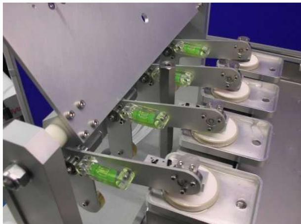
Teeth samples, which are normally set in epoxy discs, are held in radially sprung fixtures.
