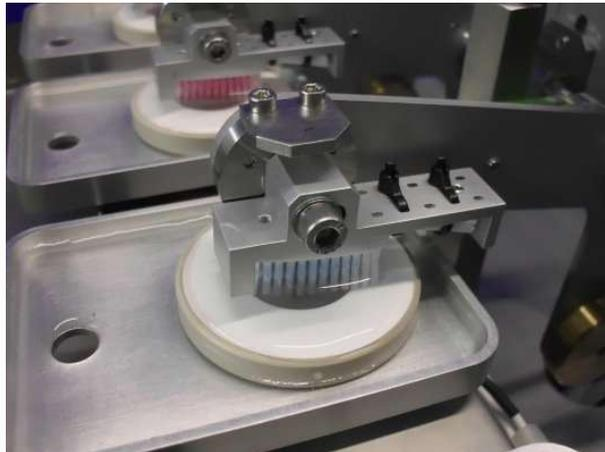
Load is applied directly to each toothbrush sample by dead-weights acting on linear bearing mounted load rods.
