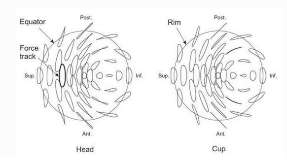
The force track on the femoral head is elliptical with an aspect ratio of 3.8, which has been shown to be a good representation of human gait. The length of the force track is 1.73r, where r is the head radius.
