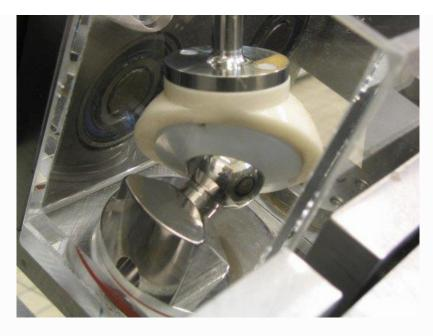
An acrylic lubricant chamber with a volume of 500 ml fits over the test components. The fluid volume is deliberately large in order to eliminate the possibility of overheating of serum-based lubricants.
